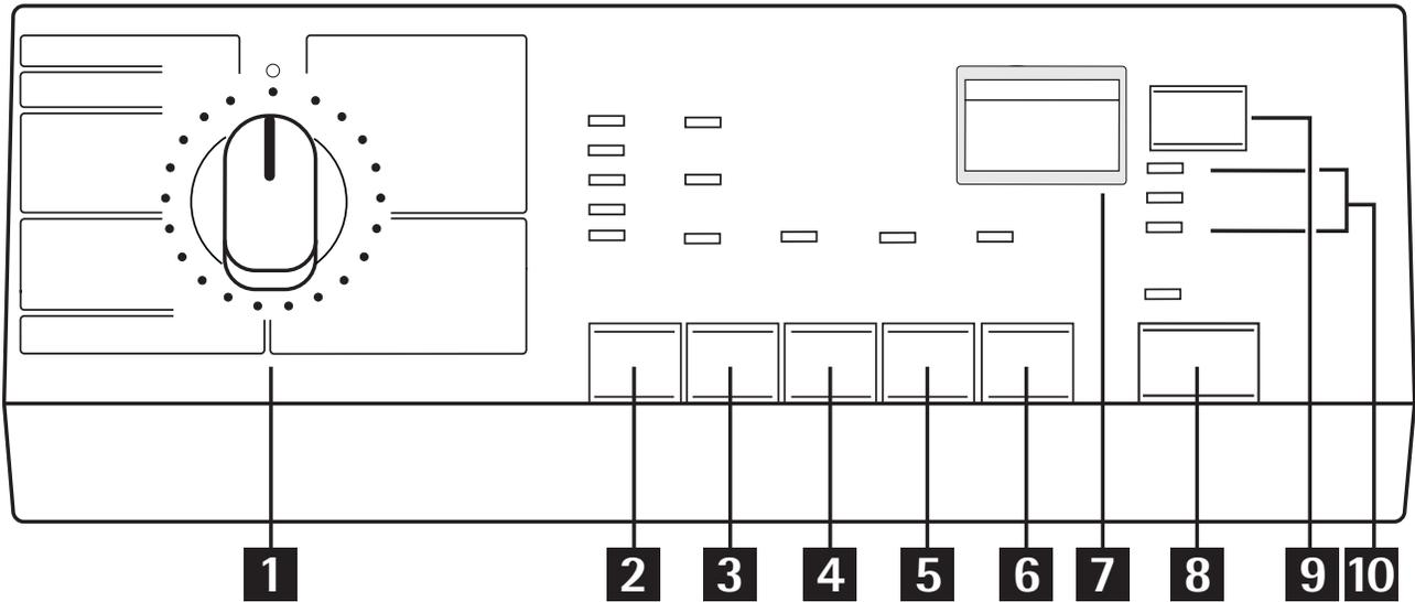
**i** The control panel is illustrated above. It shows the programme selector dial as well as the different buttons, the pilot lights and the display. These are represented by relevant numbers which are explained in the table below.
