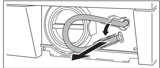
5. Release the emergency emptying hose, place it in the container and remove its cap.
