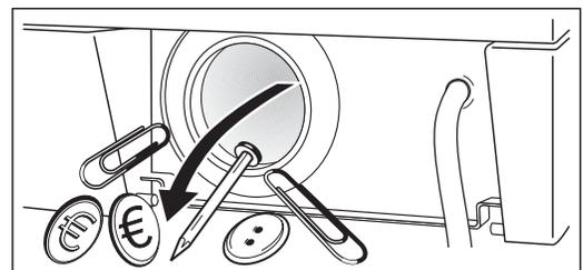
7. Remove any objects from the pump impeller by rotating it.
