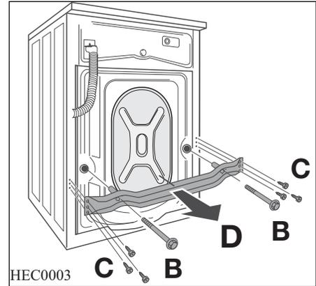
5. Remove the bracket **D** and tighten up the six smaller bolts **C**. Slide out the relevant plastic spacer **E**.
