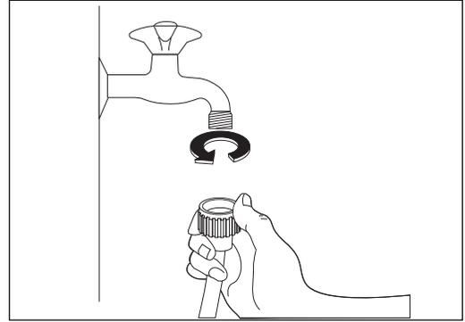
Installation should comply with local water authority and building regulations requirements. A minimum water pressure of 0.05 MPa is required for safe operation of the appliance.
